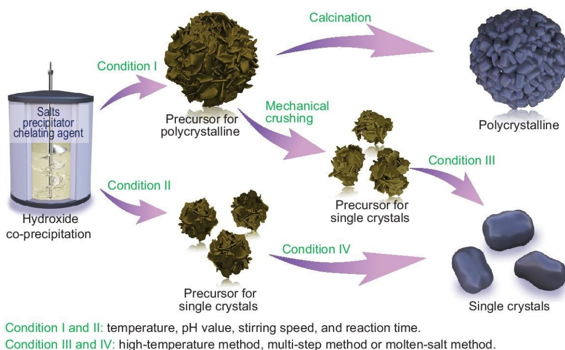
Figure 17 Synthesis Methods for SC and PC NMC cathodes [29] Copyright 2023, NSR National Science Review
