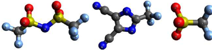
Figure 3.1: Chemical structures of the anions TFSI (bis(trifluoromethanesulfonyl)imide) (left), TDI (4,5-dicyano-2-(trifluoromethyl)imidazolid) (middle), and Tf (trifluoromethanesulfonate) (right).
