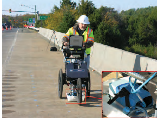
Figure 2: Ground penetrating radar testing [26].
