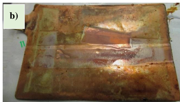
Opening pouch cells, Electrode soaked in electrolyte for 24 hours. (3 electrodes)
