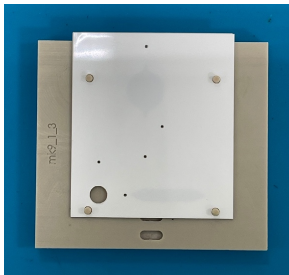
Image 1. Holder with the assembled microfluidic cassette.
