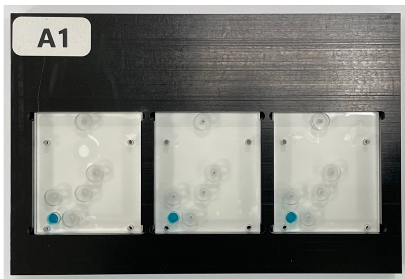
Image 7. Picture of portable holder with installed microfluidic cassettes.
