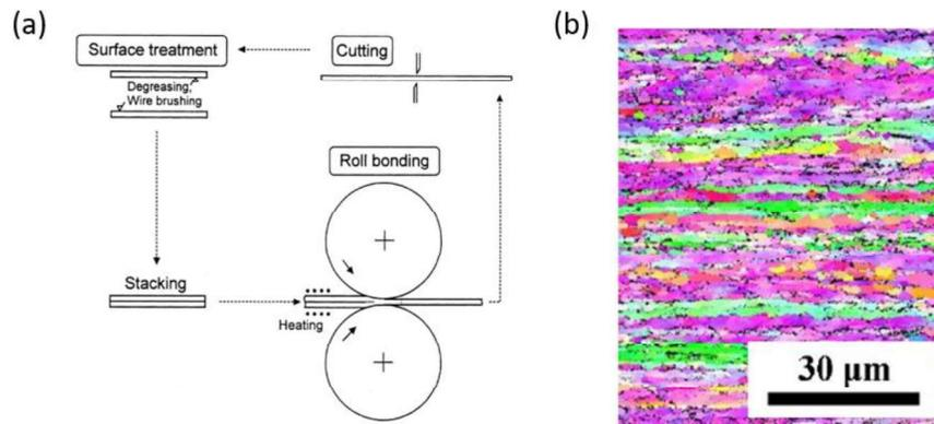
Fig. 10 Diagram of Accumulative Roll Bonding [34] (a) and microstructure of 1199 after 4 ARB passes [35] (b)
