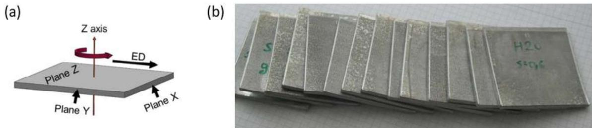
Fig. 32 Diagram of plate rotations (a) and processed plates (b)
