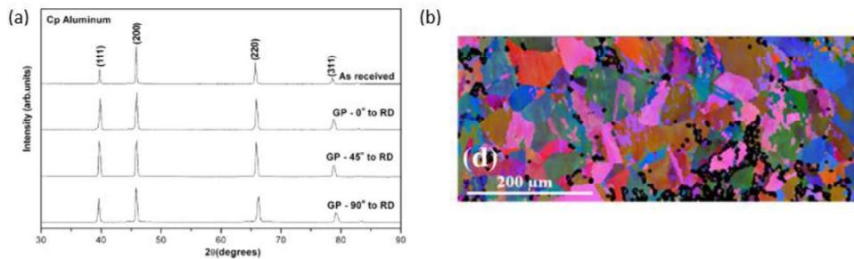
Fig. 20 Change of (111) peak intensity attributed to creating shearing texture [61] (a) and microstructure of Cu-Zn CGP pressed sheet [62] (b)
