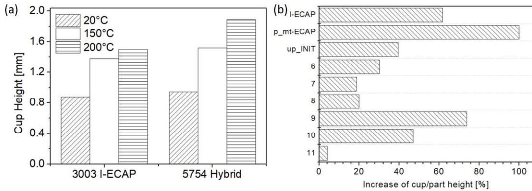
Fig. 39 Cup height of UFG 3003 and 5754 alloys investigated in the thesis, after deformation at various temperature (a) and increase in cup height formed at elevated temperature of 200°C in comparison with RT, with the exception that I-ECAPed 3003 alloy was formed at 150°C, for alloys investigated in the thesis and literature data on 5754 (samples 6-11) (b) [Appendix 3]
