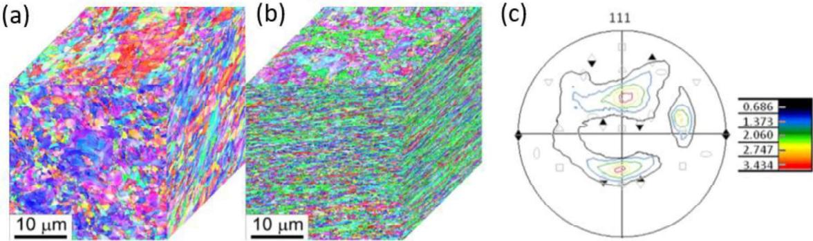
Fig. 13 Microstructure of specimen after ECAP processing (a) and subsequent rolling (b) [41] and 111 pole figure of crystallographic texture after such processing [42]
