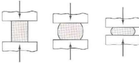
Fig. 31 Stages of upsetting process [97]
