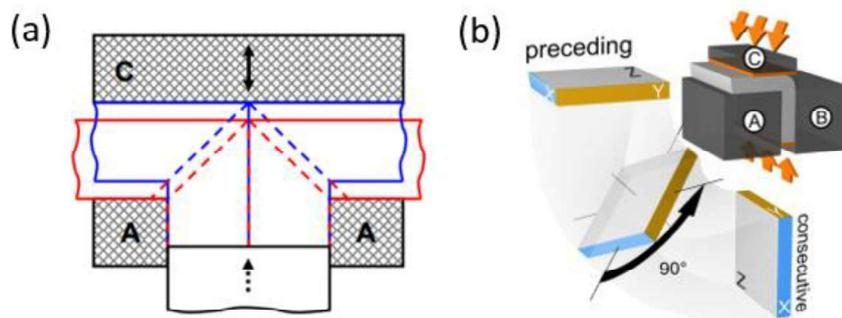
Fig. 29 Double billet I-ECAP [90] (a) and I-ECAP adjusted to plates processing [91] (b)
