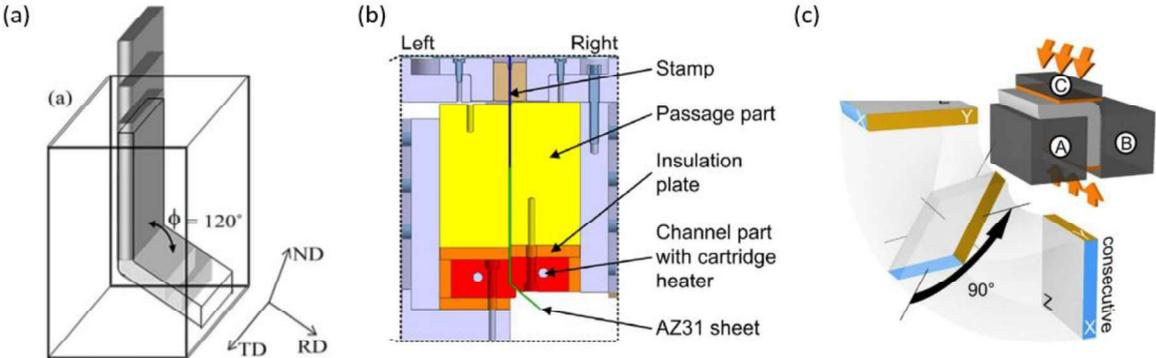
Fig. 18 Modified ECAP-based methods dedicated for sheet processing [57] (a) [58] (b) [59](c)
