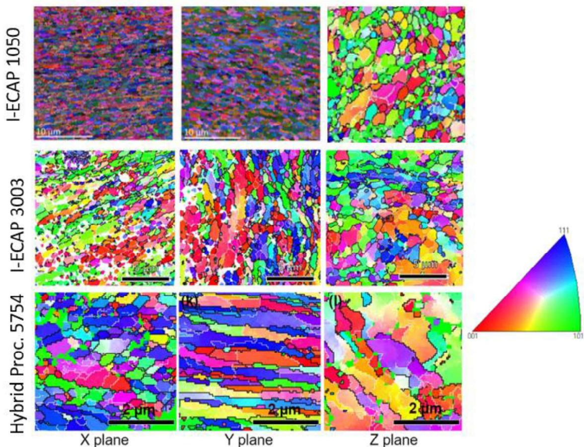
Fig. 34 EBSD maps of X, Y and Z planes of technically pure aluminum and 3003 and 5754 alloys processed by I-ECAP and hybrid method; note the various scale bars, microstructure of 1050 plane X and Y by courtesy of W. Chromiński
