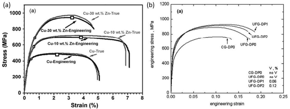
Fig. 6 Tensile curves of Cu-Zn alloy with various SFE;  $41$ ,  $22$  and  $7 \text{ mJ/m}^2$  for pure Cu, Cu-10% Zn and Cu-30% Zn, respectively [19] (a) and dual-phase carbon steel with various V content [21] (b)
