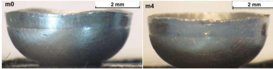
Fig. 22 Earing observed in a sheet presenting larger anisotropy (a) and reduced (b)
