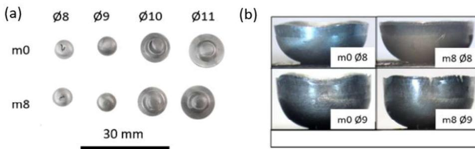
Fig. 40 Blanks drawn in cup drawing test of initial material m0 and after I-ECAP processing m8 view from top and (a) side (b)
