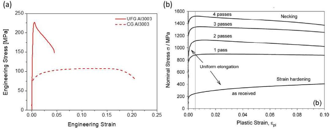
Fig. 3 Engineering stress-strain curves for UFG and CG aluminium alloy (author's results) (a), nominal stress vs plastic strain of 316L stainless steel (b) [9]
