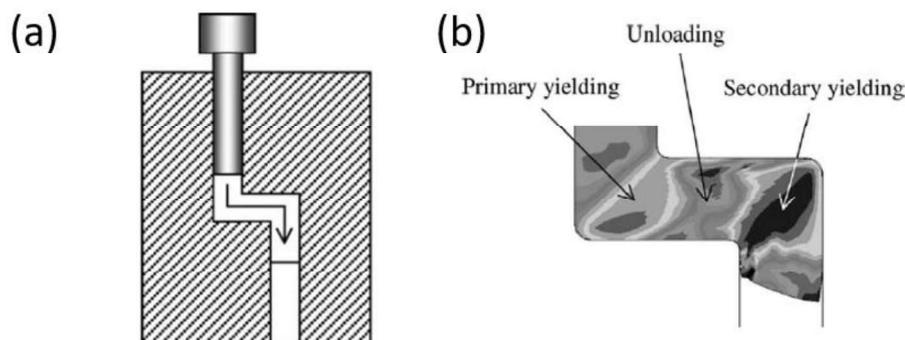
*Fig. 30 Diagram of 2-turn ECAP (a) and distribution of equivalent stress (b) [94]*
