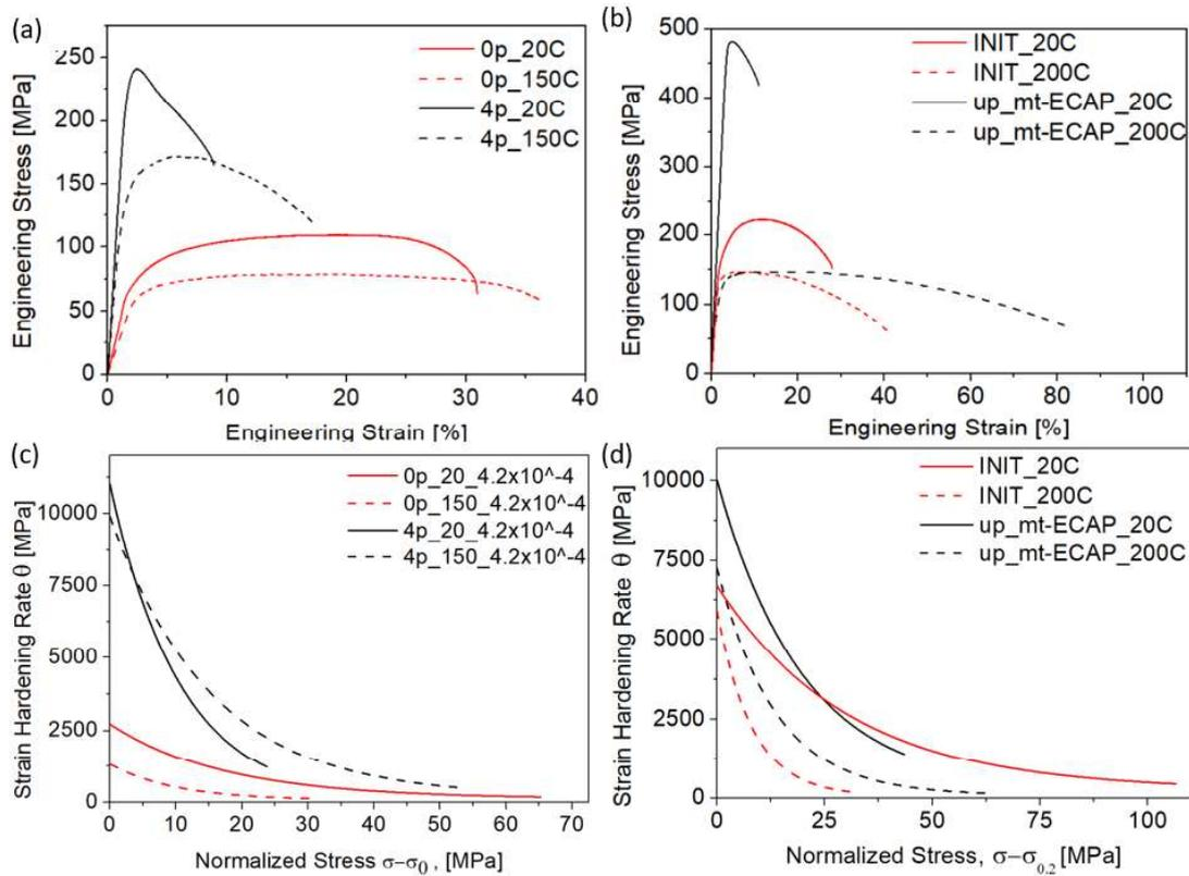
Fig. 37 Tensile curves for alloy 3003 initial material and I-ECAP processed plates (a) and 5754 alloy hybrid processed (b) and corresponding strain hardening rate curves as a function of normalized stress (c) and (d), respectively
