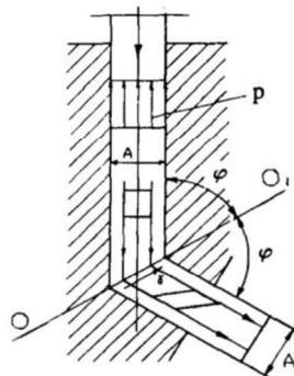
Fig. 8 Equal Channel Angular Extrusion proposed by Segal [27]
