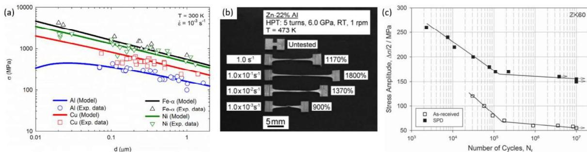
Fig. 1 Flow stress  $\sigma$  in grain size  $d$  function of various UFG metals [6] (a) and superplastic tensile specimens after deformation [7] (b), change of fatigue behavior of magnesium alloy before and after SPD processing [8]
