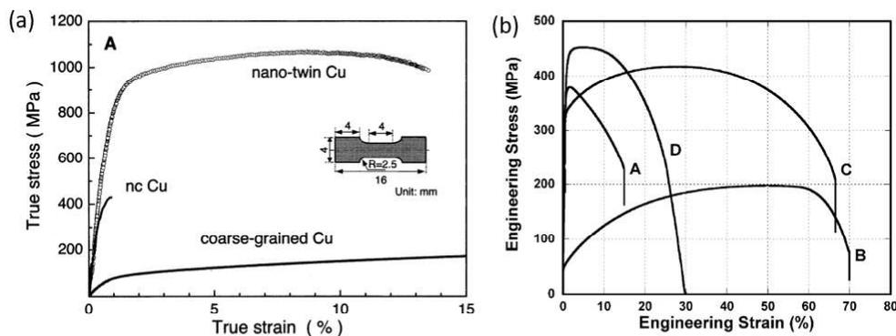
Fig. 4 Tensile curves of copper film with high density of TBs compared with nanocrystalline and coarse-grained counterparts [13] (a), Cu with different microstructures; Cu after ECAP – A; coarse grained Cu – B; bimodal nanostructured Cu – C; Cu after ECAP, cold rolling at liquid nitrogen temperature and annealed – D [15]
