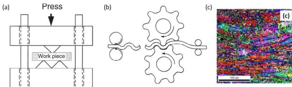
Fig. 21 Geometry of RCS tools (a), continuous RCS process (b) [63], microstructure of Al-Li alloy processed by RCS (c) [65]
