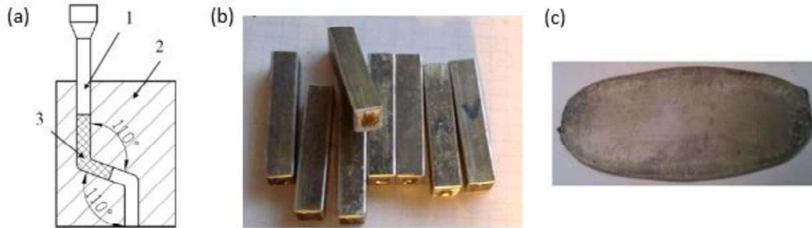
Fig. 33 Die geometry with channel curved at 110 [98] (a), mt-ECAP processed rods (b), UFG plate obtained by hybrid processing (c)
