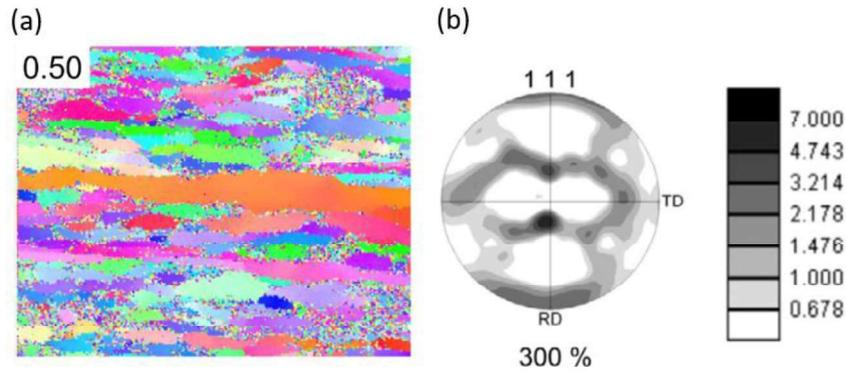
Fig. 15 Microstructure (a) and pole figure (b) of copper sample after HPT followed by rolling [44]
