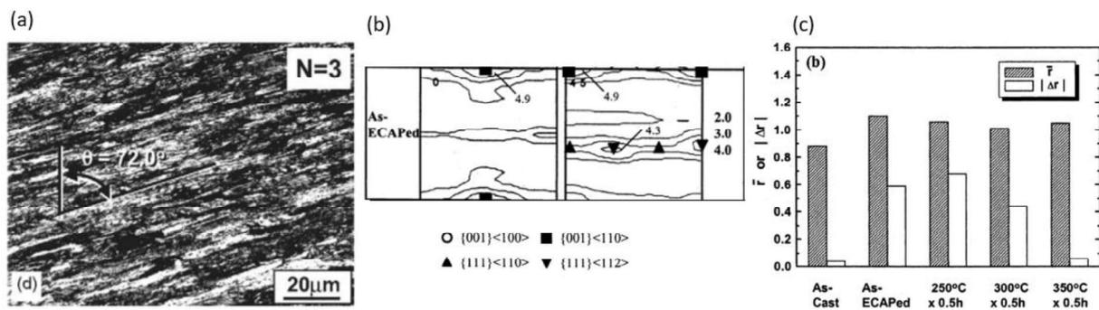
Fig. 17 Microstructure [56] (a) crystallographic texture (b) and normal and planar anisotropy [55] (c) of 1050 processed by Continuous Confined Strip Shearing
