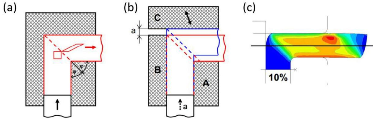
Fig. 28 Conventional (a) and Incremental (b) ECAP die, FEM simulation of I-ECAP processing with stroke value equal to 10% of billet thickness [90]
