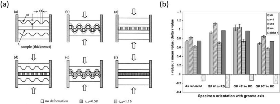
Fig. 19 Stages of Constrained Groove Pressing [60] (a) and changes of r-value for various testing direction of the material after groove pressing [61]
