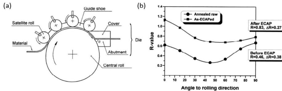
Fig. 16 Conshearing process [53] (a) and changes in R-value in a function of angle to rolling direction for aluminium sheet after ECAR process [51] (b)
