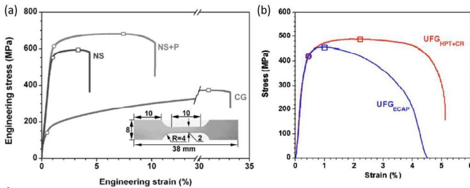
Fig. 5 Tensile curves of nanostructured aluminum (NS) and enhanced by second-phase particles (NS+P) [17] (a) and copper characterized by LAGBs with a high density of dislocations ( $UFG_{ECAP}$ ) and HAGBs with a limited number of dislocations ( $UFG_{HPT+CR}$ ) [18] (b)
