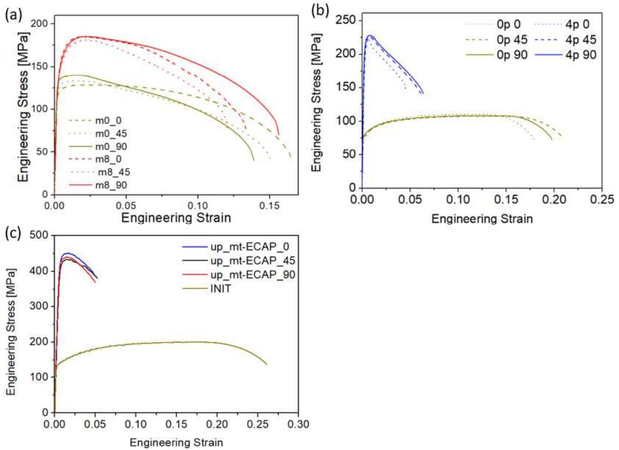
Fig. 35 Engineering stress - engineering strain of plates processed by I-ECAP, technically pure aluminium 1050 (a) and 3003 alloy (b) and hybrid method (c) cut at an angle of 0, 45 and 90° to last extrusion direction and initial material
