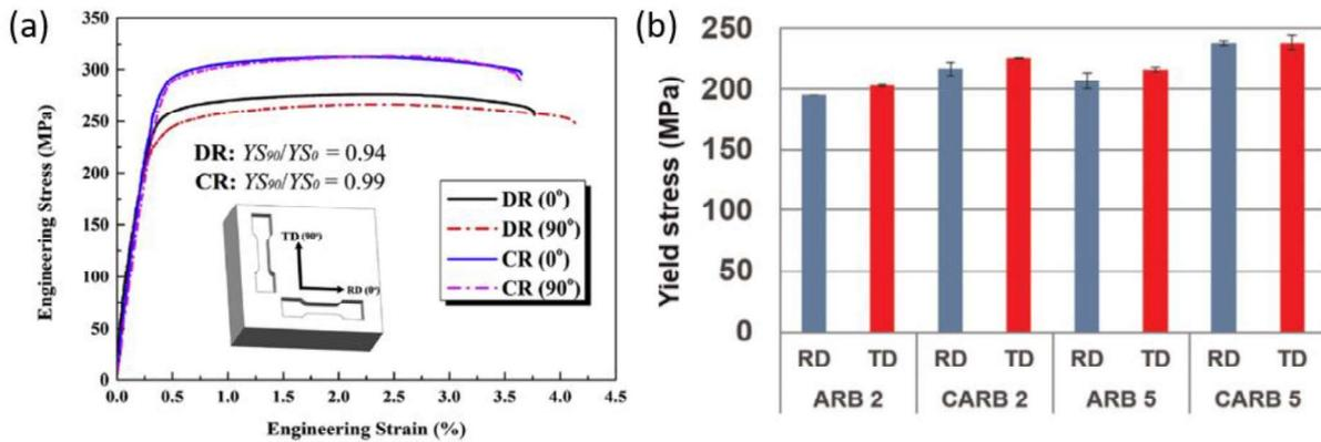
Fig. 12 Comparison of unidirectional rolling and cross rolling in ARB process in [38] (a) and [40] (b)
