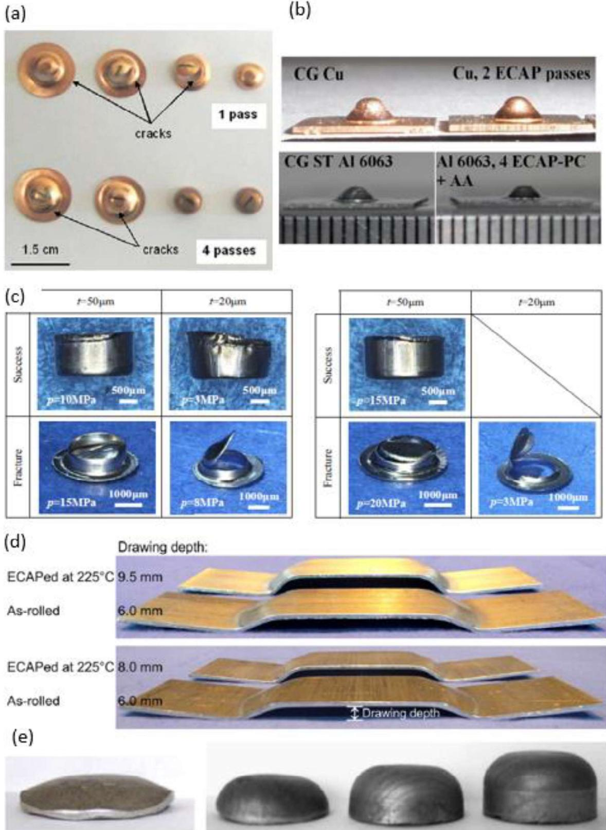
Fig. 26 Examples of forming test of UFG sheets: deep drawing of UFG copper sheet [83] (a), small punch test of UFG copper and 6063 compared with CG counterparts [84] (b), deep drawing of UFG stainless steel (left) and CG steel (right) [88] (c), U-channel forming test of CG and UFG Mg alloy [58] (d) and deep drawing of CG (left) and UFG (right) AZ31 Mg alloy [82] (e)
